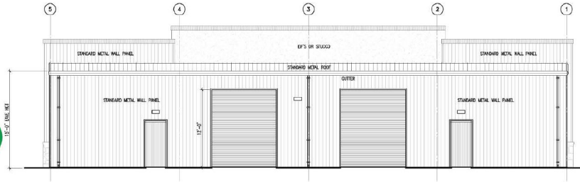
02 REAR EXTERIOR ELEVATION SCALE: 3/16"=1'-0"
